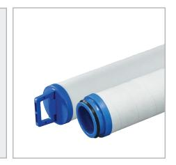
The PEACH DynaSep, Series EZ-PCHG, cartridge utilizes PEACH technology to remove deformable and shear sensitive contaminants from natural gas streams. The unique end cap design requires no tools, allowing for easy installation and removal during change-outs. The inclusion of EZ-Align® ensures a positive seal and prevents cartridge sagging. The unprecedented
